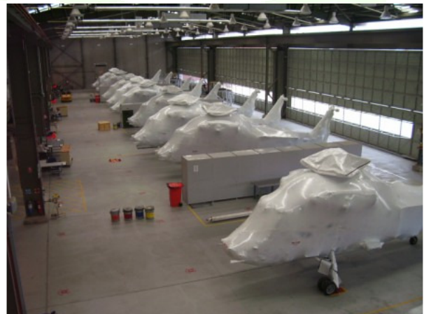
Integra wrapped and protected Sea Sprite helicopters.
